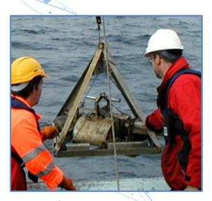
A further extended bucket lip reduces sediment washout during retrieval. The unit can be supplied with a stand allowing for easy sample access and handling. A further modification that was made provided an efficient closure system to allow arming by a single person. This modified Day grab has become the standard operating tool for the North Sea.
